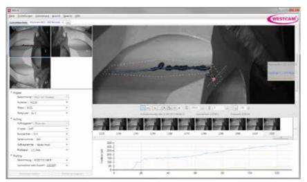
Online crack detection with crack development chart
