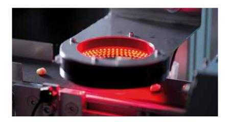
We complement your CAD / CAM process with a powerful automation solution, which dental components can assign error-free to the individual customer. This is done fully automatically by optical image acquisition and an image recognition software.
