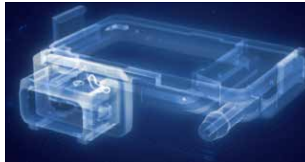
Visualization of voids on volume data
